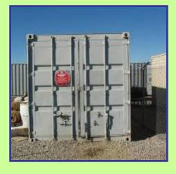
Store pesticides in a structure with a concrete pad and curb to contain spills and leaks. Locate pesticide storage and mixing areas as far away from water conveyances as possible.
