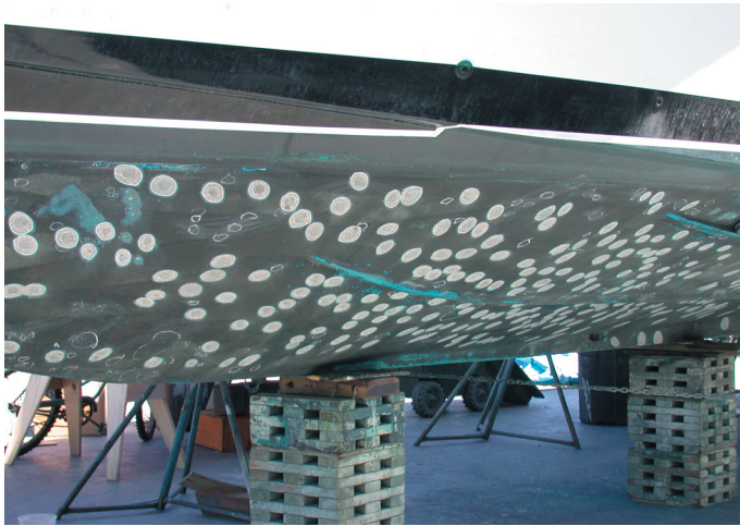
Blister Repair Job
