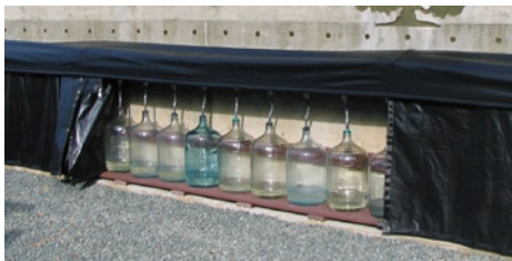
Shown here are the lysimeters' water collectors and water output from the soil profiles.
