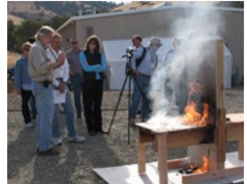
Quarles, left, shows that the plastic composite decking on the left burns more readily than the redwood on the right.
