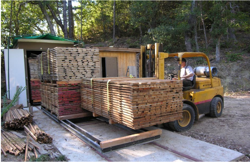
Figure 4. A track-loaded dry kiln manufactured by the Koetter Kiln Company, designed for lumber units 8 feet to 24 feet long. Kiln is shown here with 6 units of 8 foot lumber (6,000 bf capacity).
