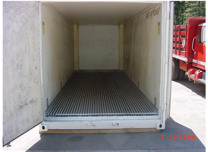
Figure 2. Insulated Shipping Container before Kiln Conversion, with Refrigeration Unit Removed.
