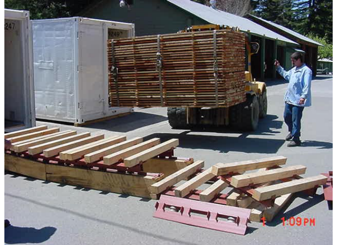
Figure 10. Loading a Unit of Lumber (4ftx5ftx8ft) onto the Kiln Cart
