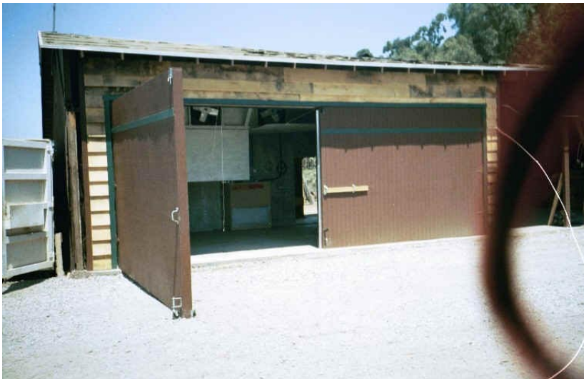
Figure 4. A track-loaded dry kiln manufactured by the Koetter Kiln Company, designed for lumber units 8 feet to 24 feet long. Kiln is shown here with 6 units of 8 foot lumber (6,000 bf capacity).
