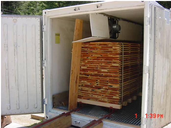
Figure 15. Loaded Kiln Ready to Close the Doors
