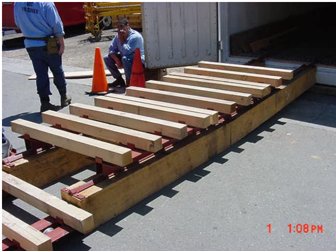
Figure 9. Empty Kiln Cart on Track Extensions
