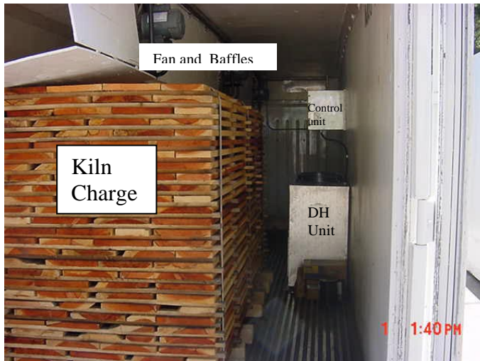
Figure 3. Inside of Completed Kiln Chamber with Charge of Lumber in Place
