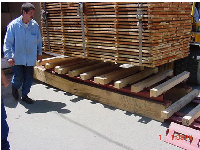
Figure 11. Placement of the Unit of Lumber on the Kiln Cart Supports
