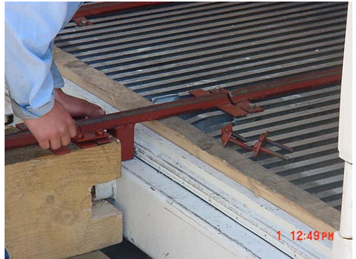
Figure 8. Close-up of Track Extension Connection to the In-kiln Tracks
